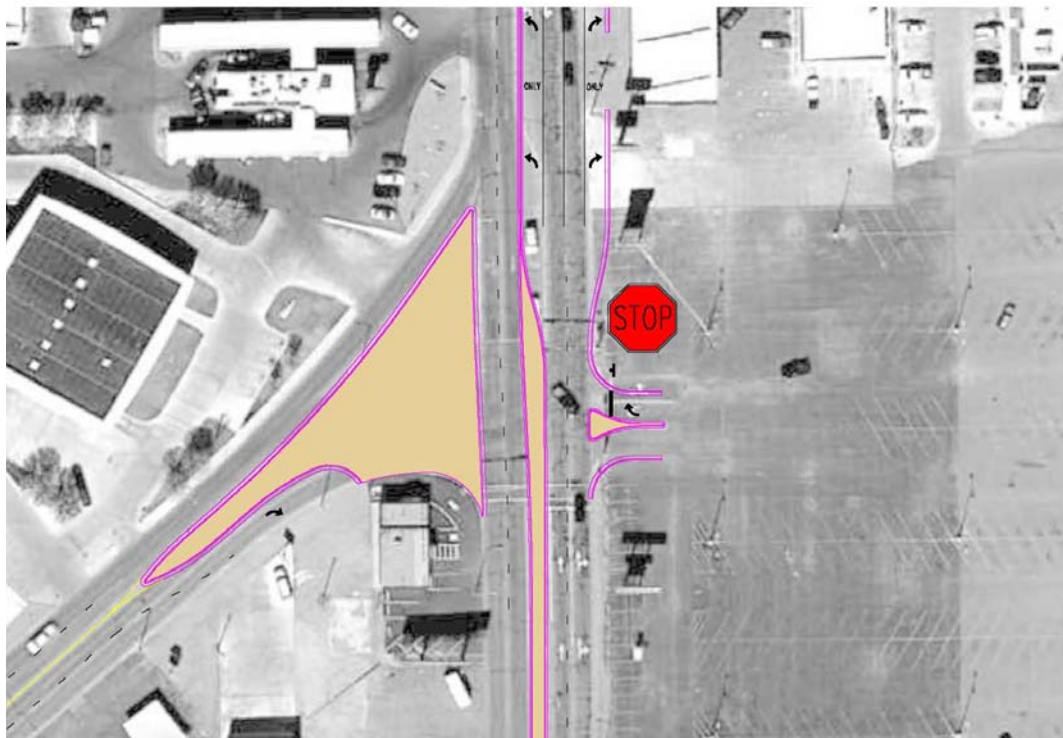
Figure 5: Alternative 3 – Westbound Right-In/Right-Out Access
